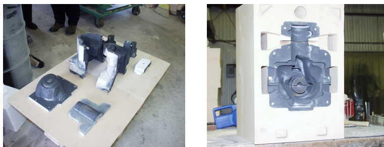
Figure 4: Shell Method – ZCast components of a shell mold (left). Assembled mold with ZCast components packed in foundry sand. Note the risers, runners and sprue have been formed in the foundry sand (right).
