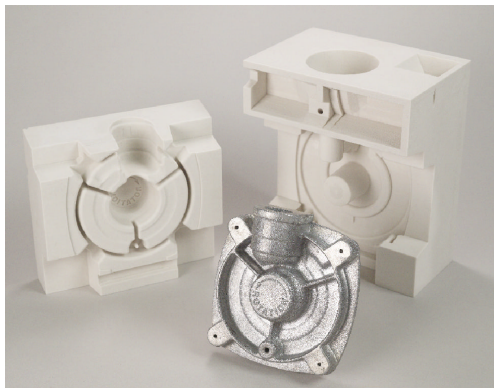
Figure 1: Cover Plate mold and casting
