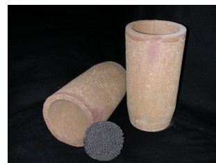
Figure 12: Refractory sleeves and filters
