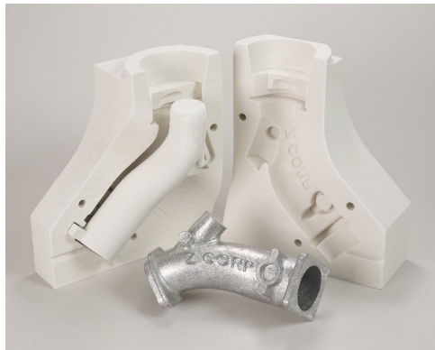
Figure 2: Manifold mold and casting
