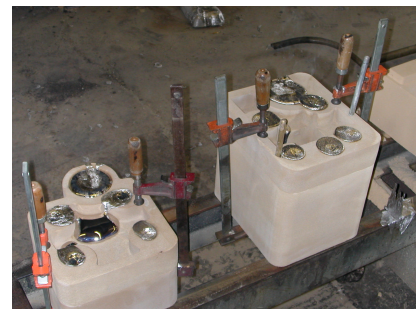
Figure 3: Direct pour molds in aluminum after pouring (note significant number of risers).
